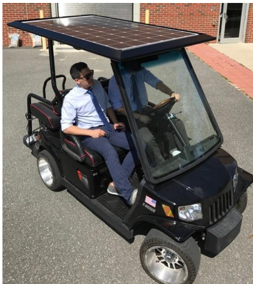
Figure 10. Electric vehicle with solar panel installed
