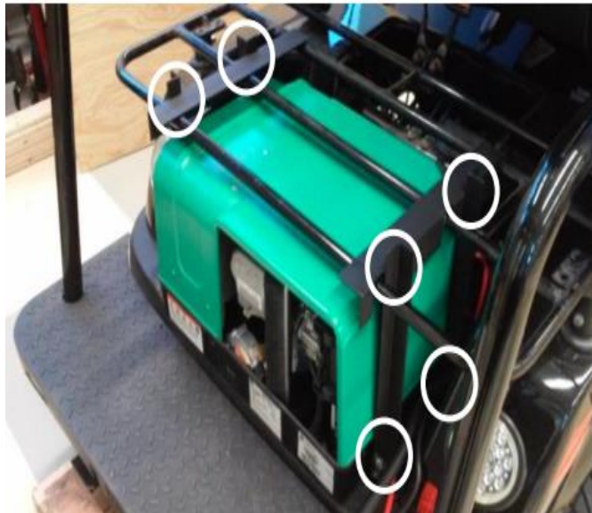
Figure 8. Generator location and mount
